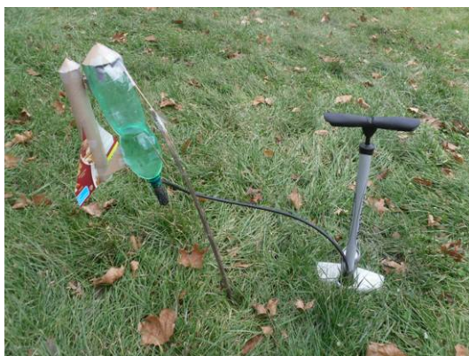
Bottle rocket assembly with the valve inserted and the space shuttle attached.
