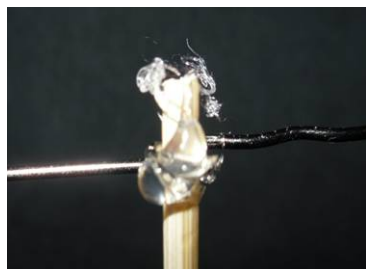
Paper clip wire and hot glue on skewer
