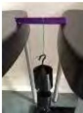
The simple beam bent and then snapped under tension. The I-beam did not bend or fail.
