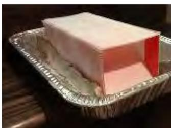
This model was created using corrugated plastic. The valve was created with the same material. Wire was used for the hinge. The sides were sealed with clay.
