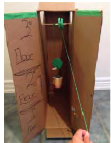
Example of an elevator model with block and tackle pulleys
