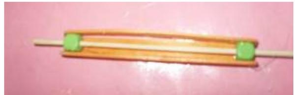
8. To build the horizontal control pivot, cut a craft stick (green craft stick in photo) in half and glue a bead (yellow bead in photo) to the rounded end of one half. Glue the other half of the craft stick to the opposite side of the bead.
