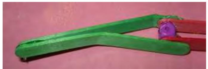
17. Build an arm extension by laying one stick flat on another one and join by gluing at one end only (green sticks in photo). Let cool. Glue together the open ends of the main section of the arm (red sticks in photo). Glue the open end of the arm extension to the glued ends of the main section of the arm (green to red sticks in photo).
