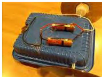
Wires connected for a parallel circuit.
