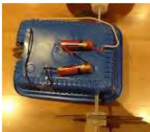
Wires connected for a series circuit.
