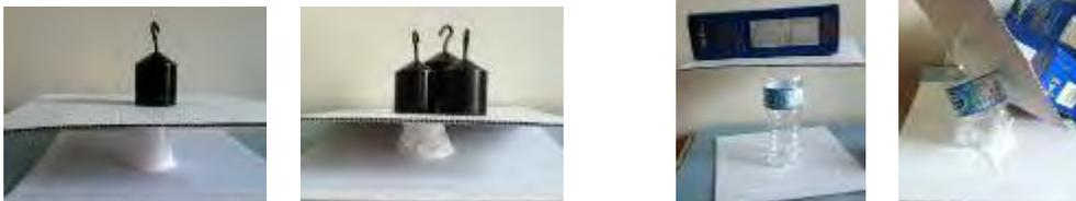
The following table illustrates sample results for the tensile and compression tests using the suggested materials. In summary, the paper plate, paper bag and licorice are stronger materials when tension is applied. The paper cup, aluminum soda can and sponge are stronger materials when they are compressed.
