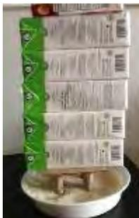
The load was made approximately 10X heavier by using 1 kg tetrapacks instead of paper back books. The tall building foundation failed with paper coin rolls crumpling once the load was 3 kg (approx. 30 books). The foundation was then built in rice (soil) and the columns strengthened by filling them with rice. The foundation could then hold 7 kg (approx. 70 books) and it eventually failed when the columns fell over (rather than crumpling).
